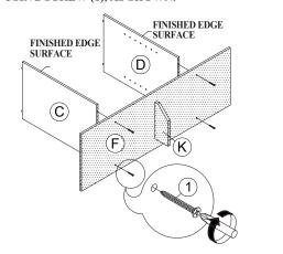
ATTACH ASSEMBLED UNIT TO TOP PANEL (A) USING GLUE (11), AS SHOWN.
