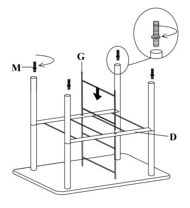
STEP 5 ATTACH MEDIUM SHELF (E) TO BOLTS (M) USING MIDDLE SPINDLES (B), MAKE SURE WIRE SHELF (G) INSERT THE HOLES OF MEDIUM SHELF (E).
