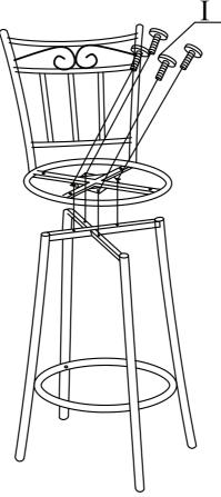
STEP 7 Attach cushion (G) onto seat frame (STEP 6) using wood screw (M) as shown.
