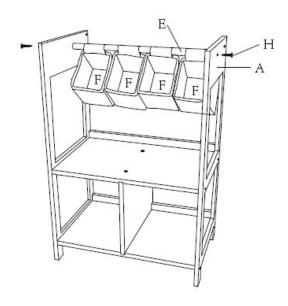
STEP: 3 Attach back panel (G) to each side panel (A) using wood screw (H) as shown.
