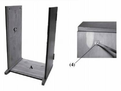
STEP 3 Insert bottom panel (B) to the groove of each front panel (C) and back panel (E) as shown.
