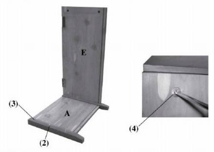
STEP: 2 Attach front panel (C) to side panel (A) using camlock pin (3), wood dowel (2) and camlock (4) as shown.
