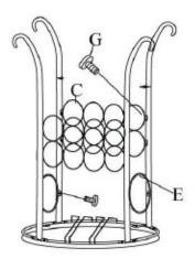
STEP 3 Attach leg connecter (D) to each legs using bolts (G), as shown.
