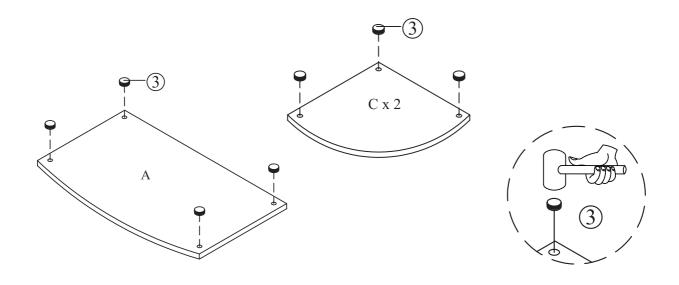
USING EITHER A SOFT RUBBER MALLET OR BY FIRMLY PRESSING THE INSERT CAPS INTO THE TOP PANEL USING THE FLAT SIDE OF A BOOK OR OTHER HARD FLAT SUREFACE TO PRESS THE CAPS INTO THE PANEL.
