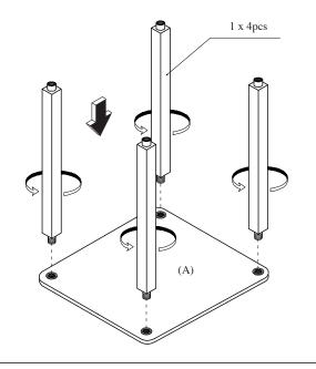
STEP 3 ATTACH SQUARE LEG (3) TO PANEL(B) AND TIGHTEN IT.
